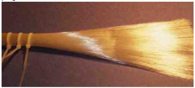
10. Fan the bundle out and shake over a garbage can to remove the shortest fibres (too short for the DFA 100 Macro - may be fine to keep with a different lens.)
