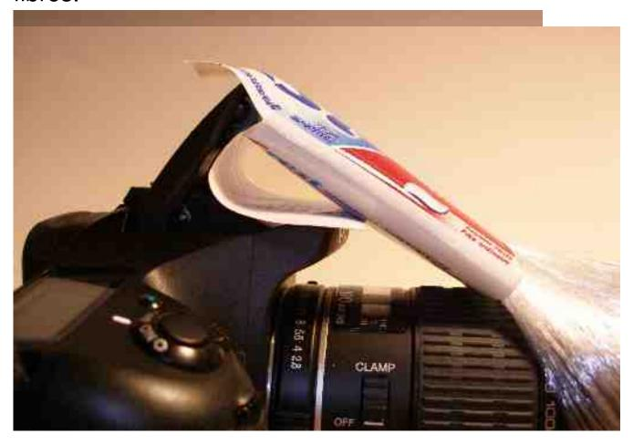
The reflective surface inside the tube directs the light into the fibres. A gentle curl of tube over and under the pop-up flash will hold it nicely in place.
