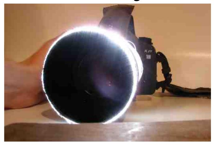
This is a fibre-optic flash extension for your DSLR's popup flash. Totally easy! Works great! Durable! Designed specifically for K20D with 100 2.8 DFA lens but adaptable to other lenses (see Tamron Adaptall 90 2.5 example at the end.) Build your own!
