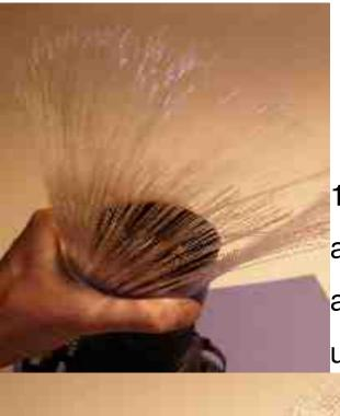
17. Use a section of balloon to anchor the fanned-out fibres around the lens hood. (Roll it up from below.)
