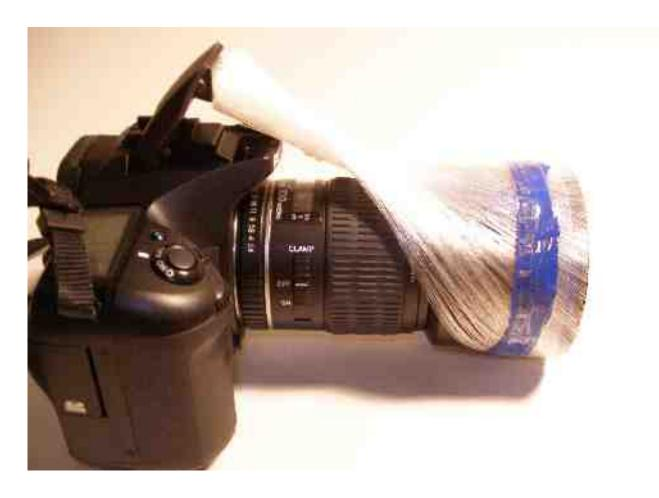
21. Get your last fresh fibre-optic bundle. Cable-tie the tip so that the longest fibres are kept.
