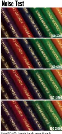
Upto ISO 400, there is barely any noticeable difference. Noise creeps in at ISO 800 and slowly increases. Dynamic range begins to visibly reduce at ISO 3200. Images are printable well at full size (about 20  $\times$  30 inches), with minimal noise reduction, till ISO 3200. While I would not recommend moving beyond ISO 25,600, the linearity of the deterioration allows you to retain quality and colour by halving the image size for every progressive stop after ISO 3200.
