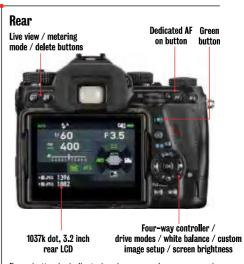
Every button is dedicated and many can be repurposed. With the 'green' button, you can instantly reset exposure to the chosen 'Program Line' behaviour, making shutter and aperture priority, and the program mode instantly accessible without really using the exposure mode dial.
