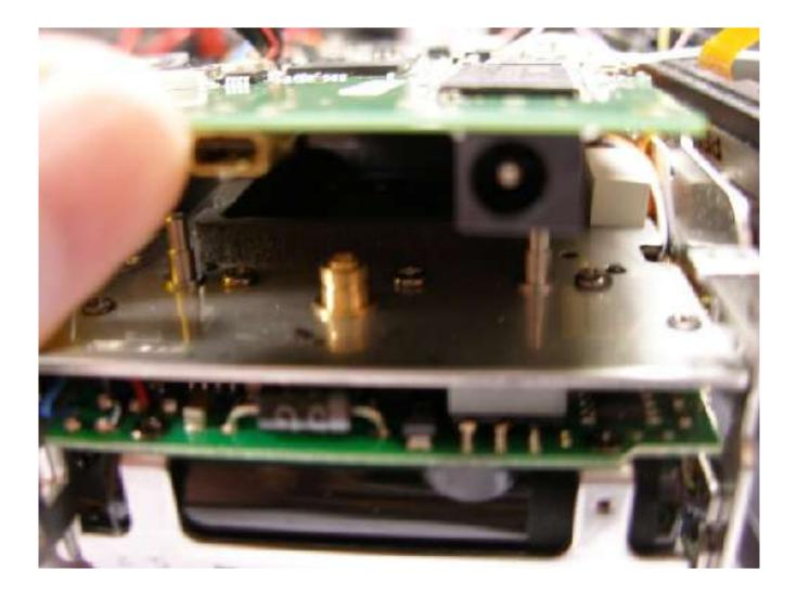
Takes a bit of wiggling - but you don't have to cut any wires to get the sensor out.
