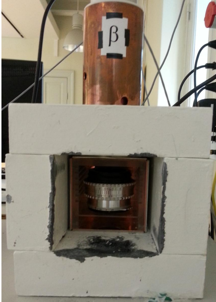
Figure 3: The setup for the beta measurement of the Carl Zess Tessar objective. The measurement chamber consists of 5 cm lead in order to shield from the external background radiation.
