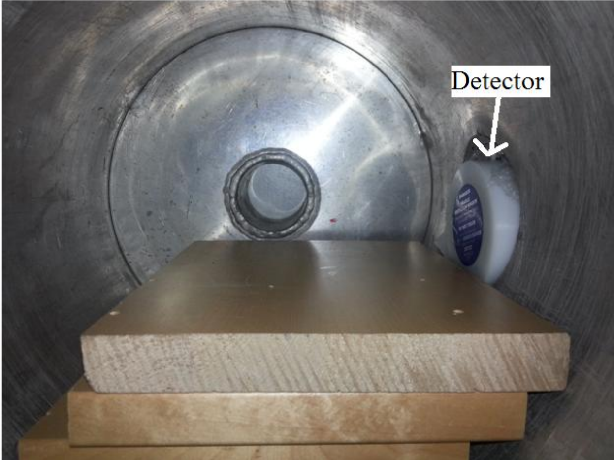
Figure 2: Inside the gamma measurement chamber. The front end of the detector is marked on the right in the image. The walls of the measurement chamber include a 5cm lead layer, shielding against the surrounding natural background gamma ray radiation.
